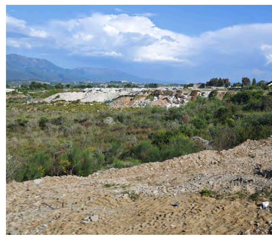
Fill consisting of a mixture of rubble and waste along riverbanks for urbanization.
